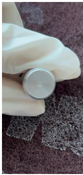
Abrasion of dolly and composite surface
