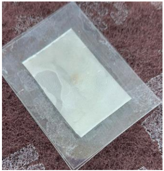
Abrasion of dolly and composite surface
