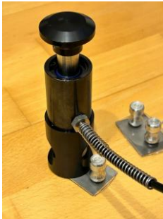
Attach actuator onto dolly
