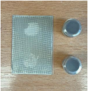
Composite and dolly surface after the pull-off test
