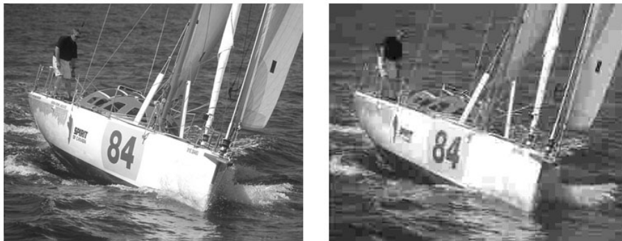
Figure 2: Test image for objective PQE a) reference picture (non-compressed static picture), b) degraded picture (DCT based compressed I-frame MPEG-2).
